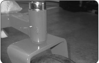
There is one grease fitting on each of the actuator bar pillow blocks located under the fuel tanks. Grease twice a season.
